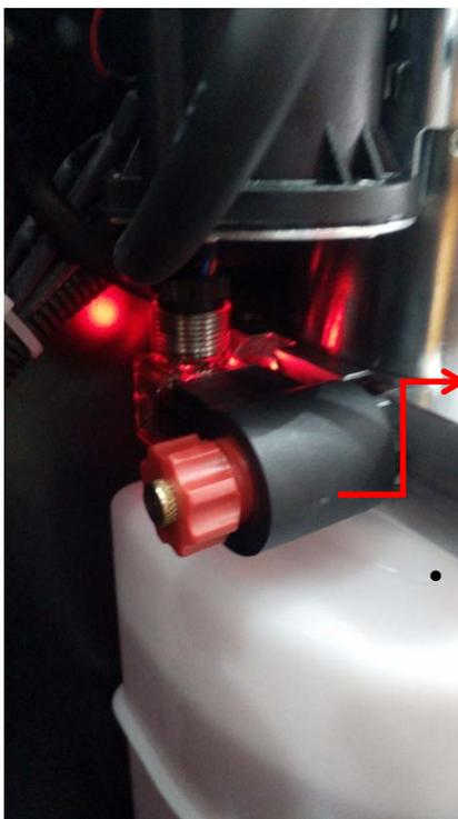
1. If the vehicle cannot be lifted normally, for example, the original 3300 lbs. vehicle can only be lifted less than 2200 lbs., then the oil pump pressure can be adjusted, but this operation must be carefully, if the hydraulic pressure is adjusted so that the vehicle load exceeds the rated, it may make the frame deformation. Specific operations are as follows:
