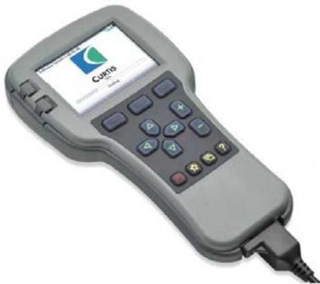
**Warning:** The control system can affect the vehicle's acceleration rate, deceleration rate, hydraulic system and braking. A dangerous situation can occur if the vehicle control system is not programmed correctly or exceeds safety. Only the vehicle manufacturer or an authorized service agent can program the control system
