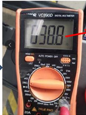
Normally, it should be about 40  $\omega$ . If no resistance is displayed, there is a problem with the brake line or a short circuit of the brake coil.
