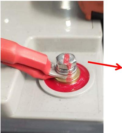
Check whether the cable connection (including other secured parts) is loose
