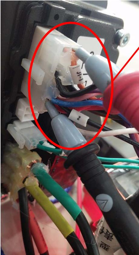
Switch the multimeter to 20V DC, insert the pen j1-1 (accelerator 0-5V speed signal) and 2 (negative pole) respectively, turn the accelerator after power on, and
